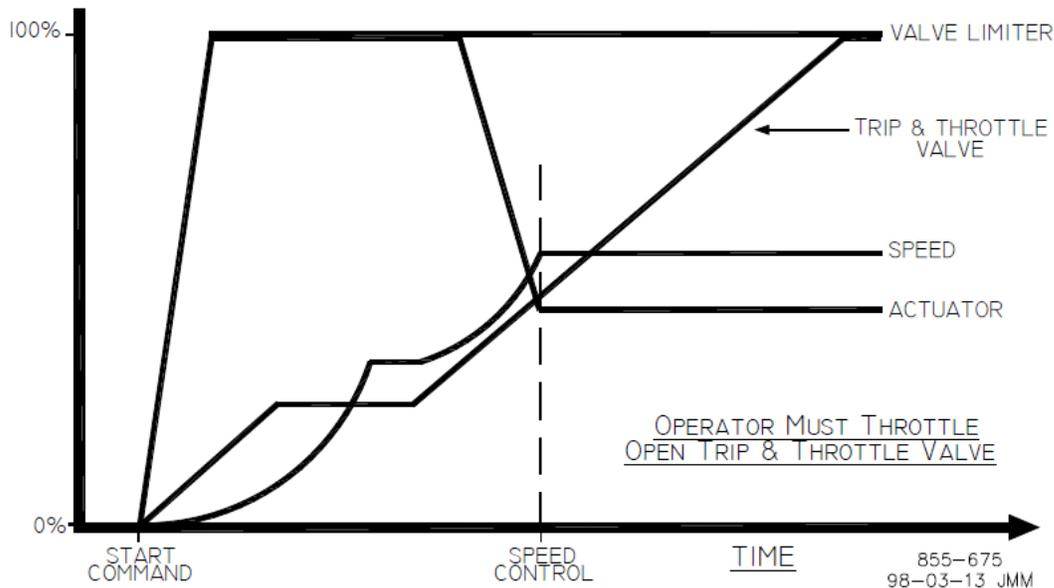
Figure 3-6. Manual Start Mode Example
