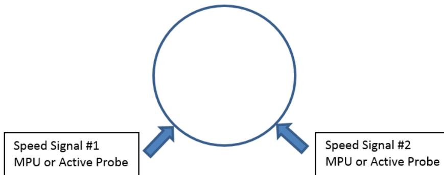
Figure 3-2. Speed Probe Mounting for Detection Test
