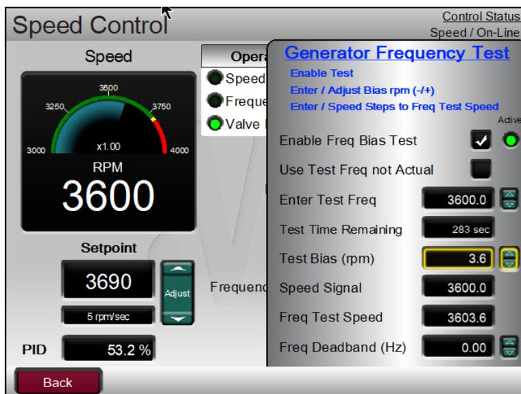
Figure 5-39. Generator Frequency Test “Active” LED Screen
