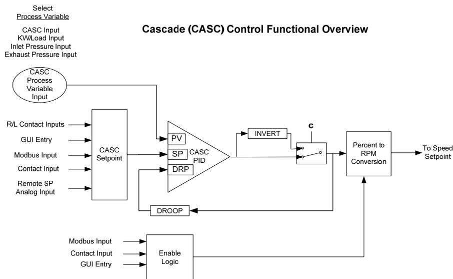
Figure 3-17. Cascade Functional Diagram
