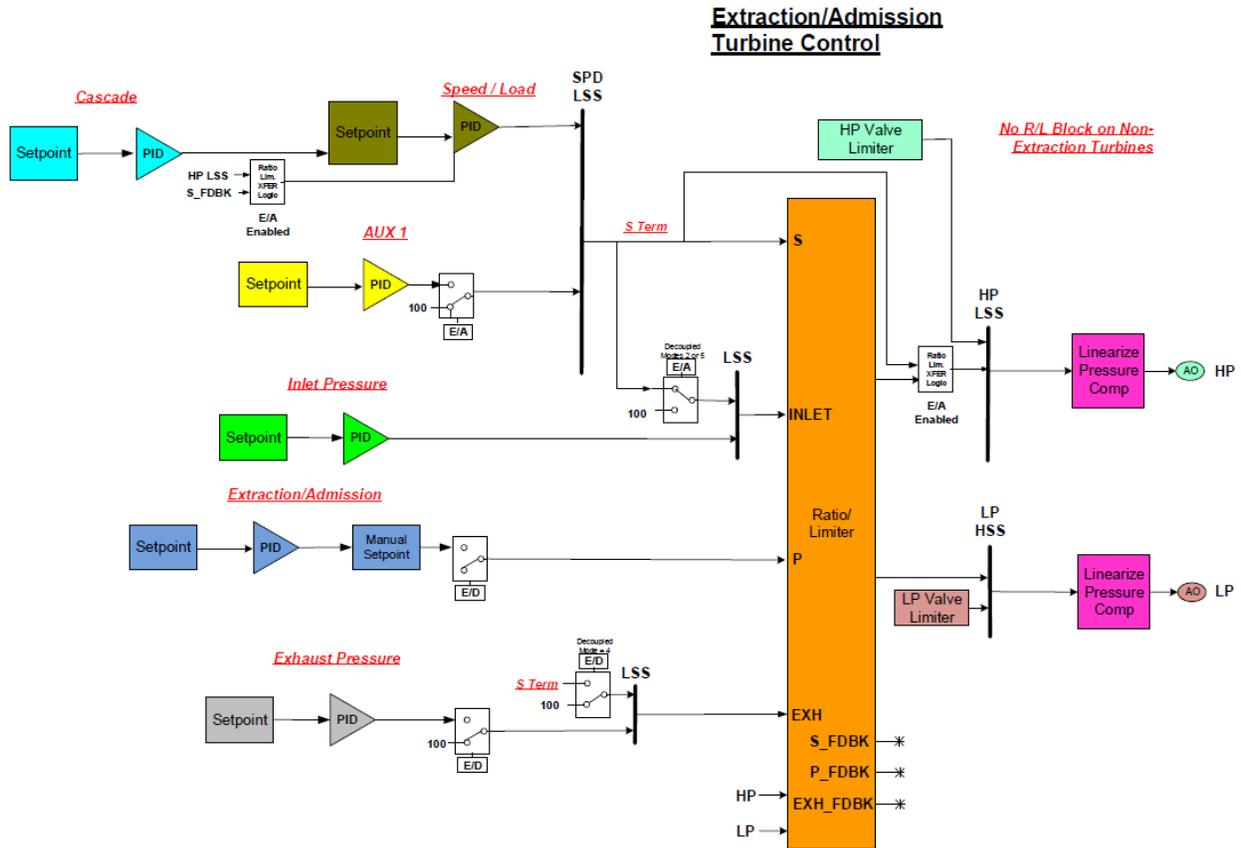
Figure 1-5. Turbine Configurations Using Extraction and/or Admission
