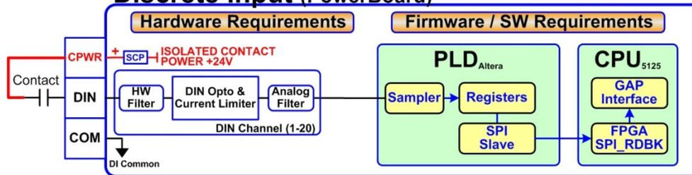
Figure 2-11. Discrete Input Block Diagram
