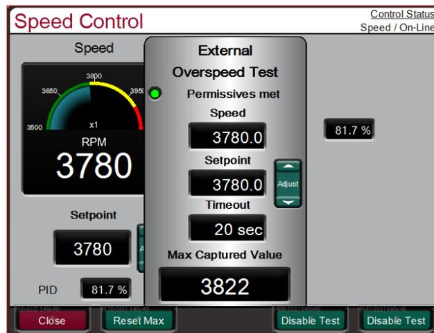
Figure 5-29. External Overspeed Test
