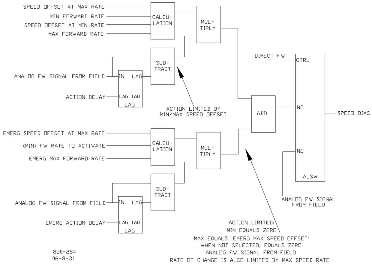
Figure 3-16. Typical Anti-surge Valve and Speed Feed-Forward Logic Trend
