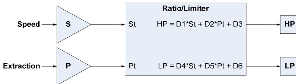
$$\begin{aligned} \text{HP} &= D1.St + D2.Pt + D3 \\ \text{LP} &= D4.St + D5.Pt + D6 \end{aligned}$$
