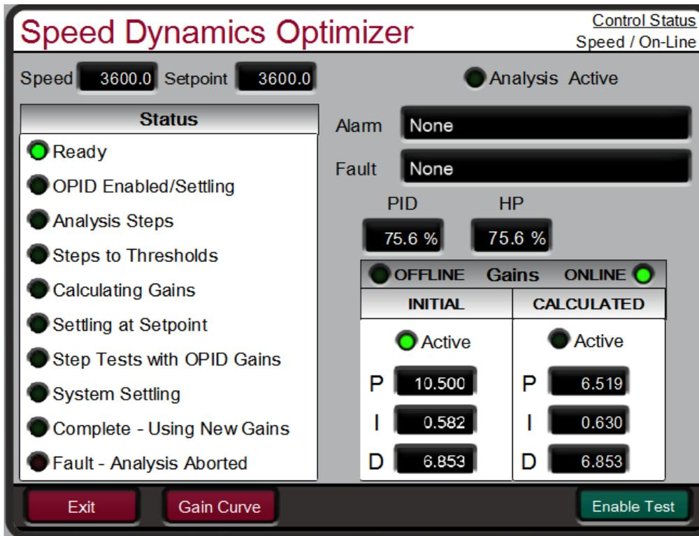
Figure 5-34. Overview of the Automated PID Optimizer Routine
