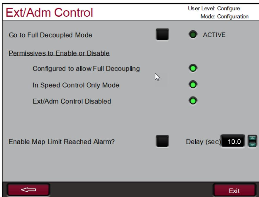
Figure 3-27. Configured for Full Decoupled Mode (No Map)
