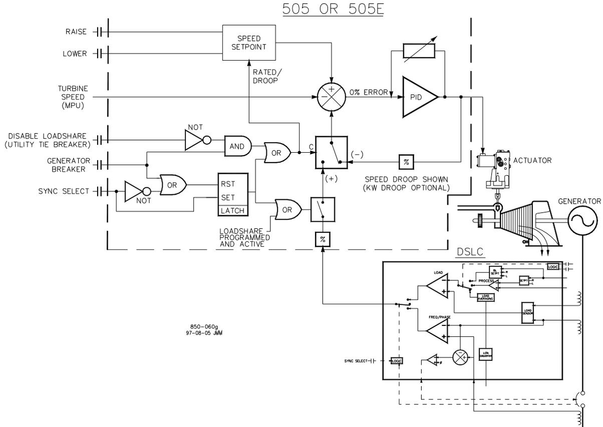
Figure 3-15. Load Sharing Logic
