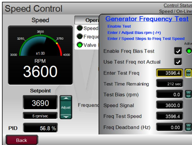
Figure 5-41. Generator Frequency Test PID Amount Increased
