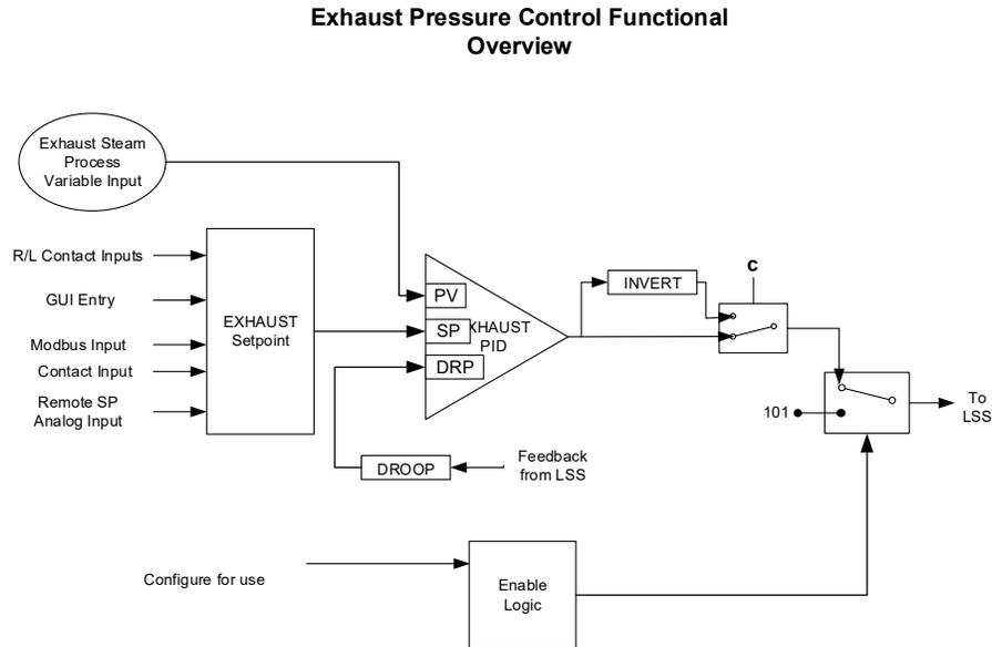
Figure 3-29. Exhaust Steam Pressure Control Overview
