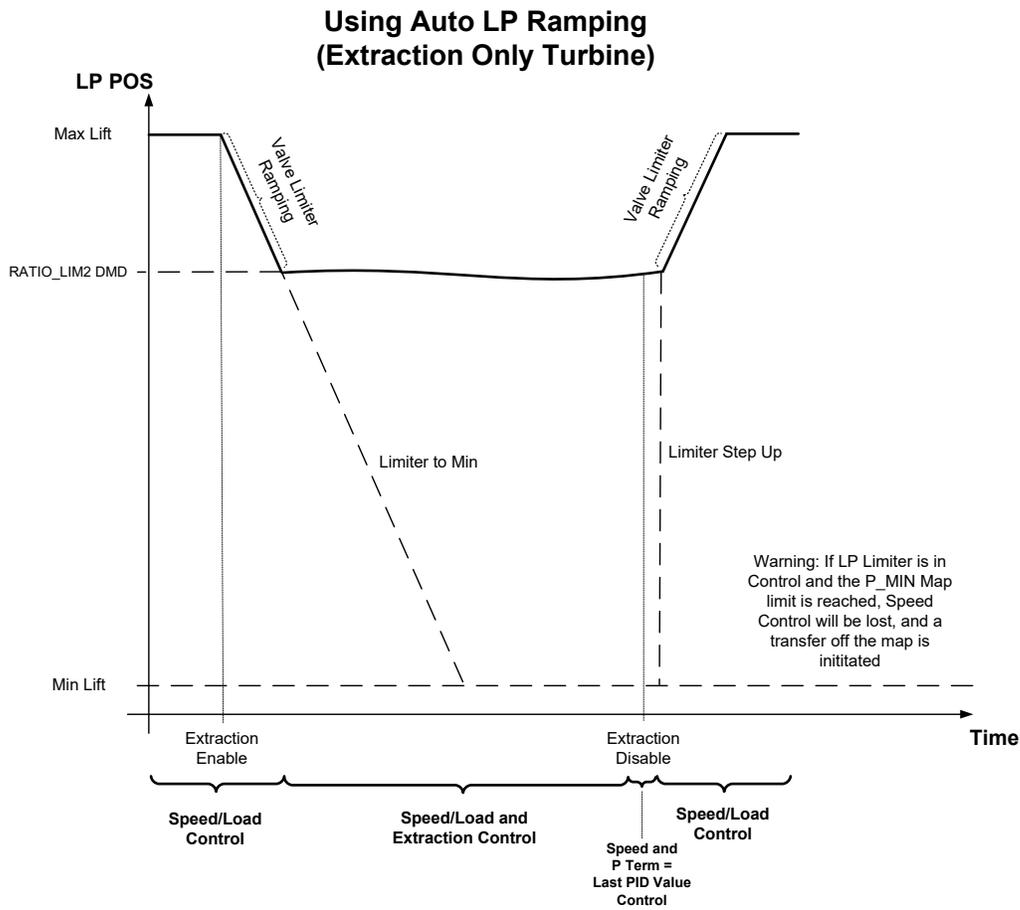
Figure 3-20. Transitions Between Speed Only and Ratio Limiter Control – Auto Mode
