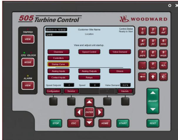
Figure 5-26. HOME Menu Showing “Startup Curve” IN-Focus
