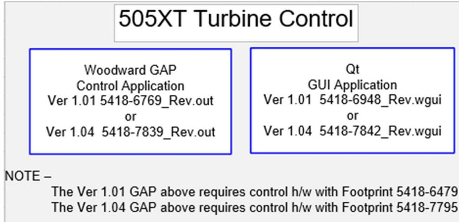
Figure 5-1. Software Architecture
