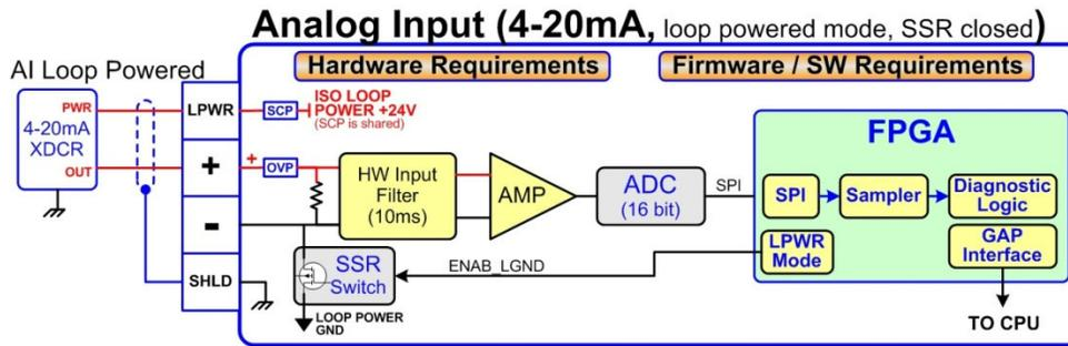
Figure 2-8. Analog Input – Loop-Powered Block Diagram
