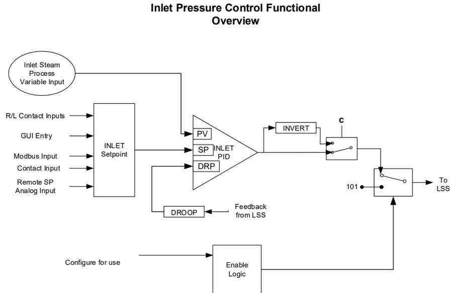
Figure 3-28. Inlet Steam Pressure Control Overview
