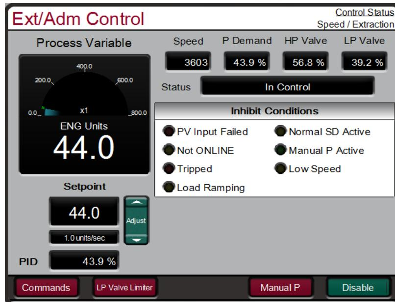
Figure 3-22. Extraction/Admission Control Panel
