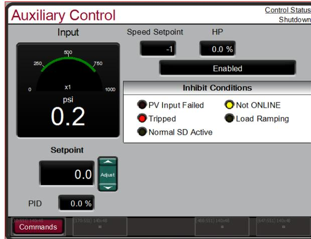
Figure 5-15. Auxiliary Control Screen
